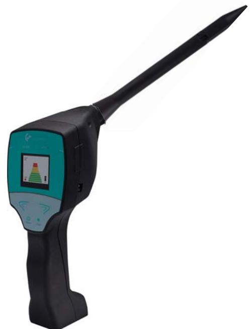
**LD 400** with focus tube and focus tip for precise locating.
